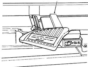
5. Hold cutterhead pulley firmly with one hand and loosen lockscrews in each wedge using a 5/32 in. setscrew wrench.
